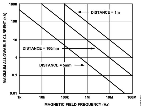
Figure 18. Maximum Allowable Current for Various Current-to-ADuM5230 Spacings
