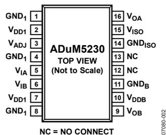
Figure 3. Pin Configuration
