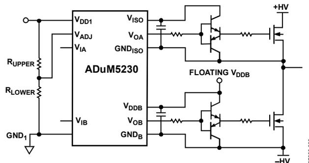
Figure 25. Application Circuit
