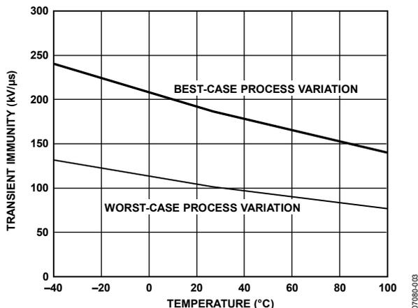
Figure 22. Transient Immunity (Linear Transients) vs. Temperature
