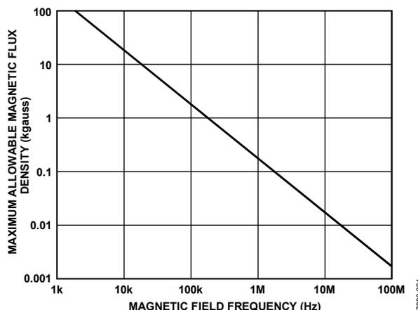
Figure 17. Maximum Allowable External Magnetic Flux Density
