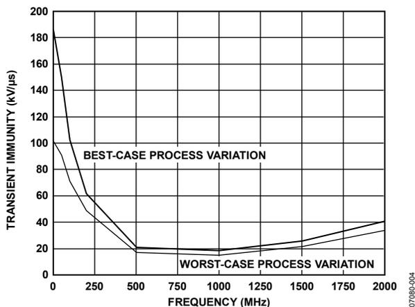
Figure 23. Transient Immunity (Sinusoidal Transients), 27°C Ambient Temperature
