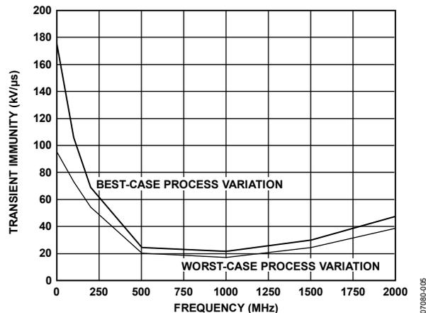
Figure 24. Transient Immunity (Sinusoidal Transients), 100°C Ambient Temperature
