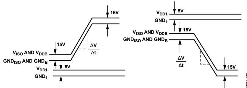
Figure 19. Common-Mode Transient Immunity Waveforms—Input to Output
